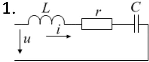
$$z = r + j\omega L + \frac{1}{j\omega C} = r + j\left(\omega L - \frac{1}{\omega C}\right)$$
