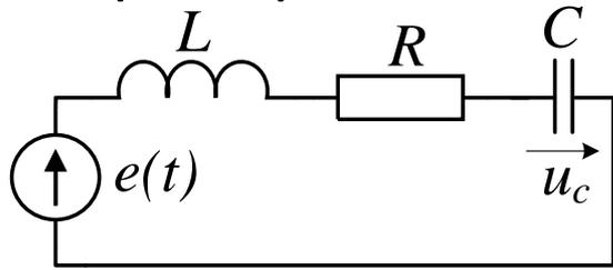
$$\left. \begin{aligned} L \frac{di}{dt} + Ri + u_c &= e(t) \\ i &= C \frac{du_c}{dt} \end{aligned} \right\} LC \frac{d^2 u_c}{dt^2} + RC \frac{du_c}{dt} + u_c = e(t)$$
