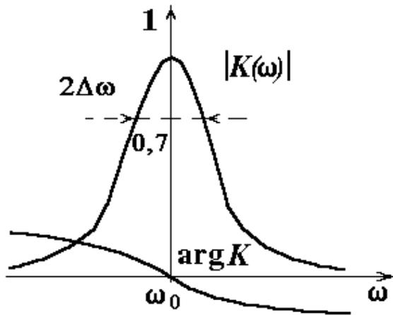
$$K(j\omega) = \frac{K_0}{1 + jQ\left(\frac{\omega}{\omega_0} - \frac{\omega_0}{\omega}\right)} = \frac{K_0}{1 + j\xi}$$
